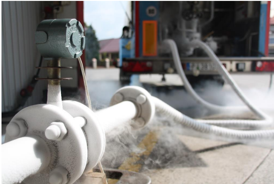
Figure 9.2: Mechanical oscillator flowmeter during the measurement of liquid nitrogen.
