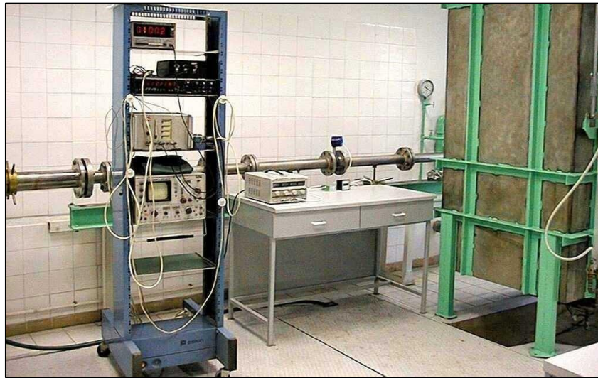
Figure 4.5: Water calibration stand with an installed mechanical oscillator flowmeter.
