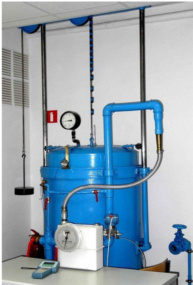
Figure 4.9: Bell prover calibration stand.
