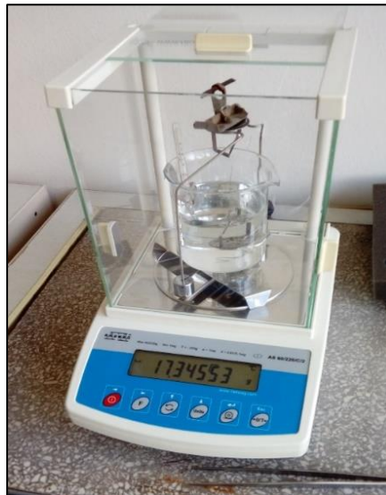
Figure 4.2: Measurement of oscillator's density.
