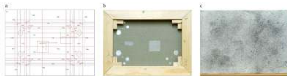
Figure 2. Model painting on canvas repaired with various methods; a: template showing positions of discontinuities introduced to the canvas and used further as a reference for analysis of the data extracted from DIC records; b: reverse with inserts and patches; c: face of the painting with a random pattern
