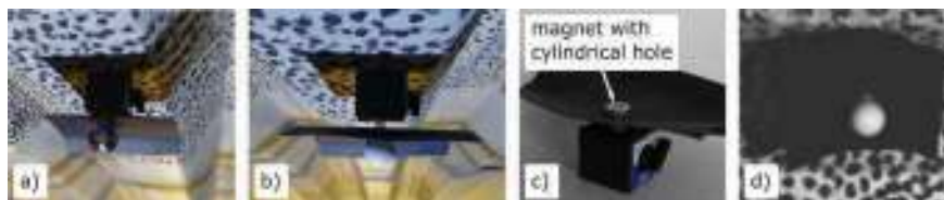
Fig. 3. Fiducial markers: a) optical target, b) ball bearing painted white matt, c) magnetic holder with a cylindrical hole for fiducial markers, d) a fragment of image with ball bearing captured by one of cameras.
