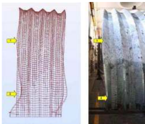
Fig. 17 Views of the model and the object during the experiment; the mesh grid of the model has been rescaled for better visualization, original mesh was finer (it contained 4176 finite elements)
