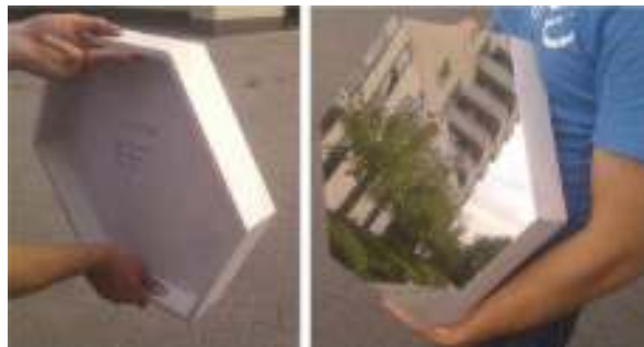
Fig. 1 The composite mirror prototype – rear and front side
