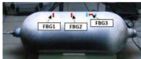
Fig. 4. Type IV vessel for hydrogen storage with marked localization of the installed FBG sensors.
