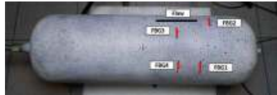
Fig. 3. The tested vessel CNG-4 type with marks indicating the localization of a flaw and the installed FBG sensor.
