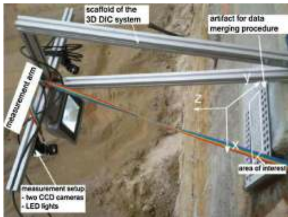
Fig. 5. View of the measurement setup and location of AoI2.
