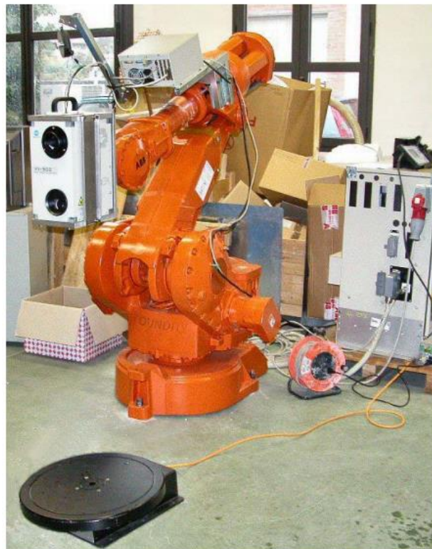
Figure 17. RoboScan system (image source (Callieri, et al., 2004)).
