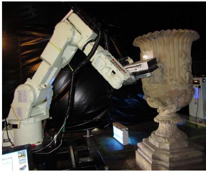
Figure 45. Garden vases scanning: a) vase in the garden of Wilanow Museum; b) tent used to provide darkness and climate control; c) vase inside the tent; d) system during measurement.
