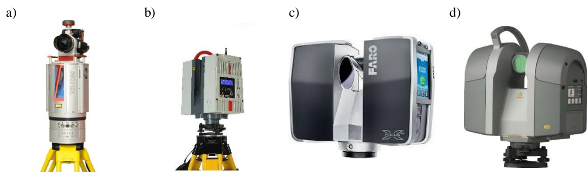
Figure 32. Time of flight scanners: a) Riegl VZ1000, b) Leica HDS; c) Faro Focus 3D; Trimble TX8 (images sources: manufacturers webpage).
