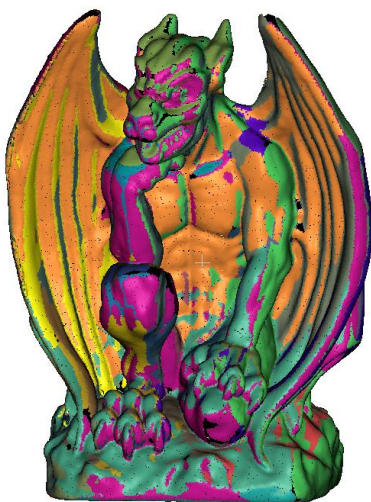
Figure 93. Results of NBV calculations for Gargoyle sculpture: a) similarly oriented areas; b) calculated scanner poses.
