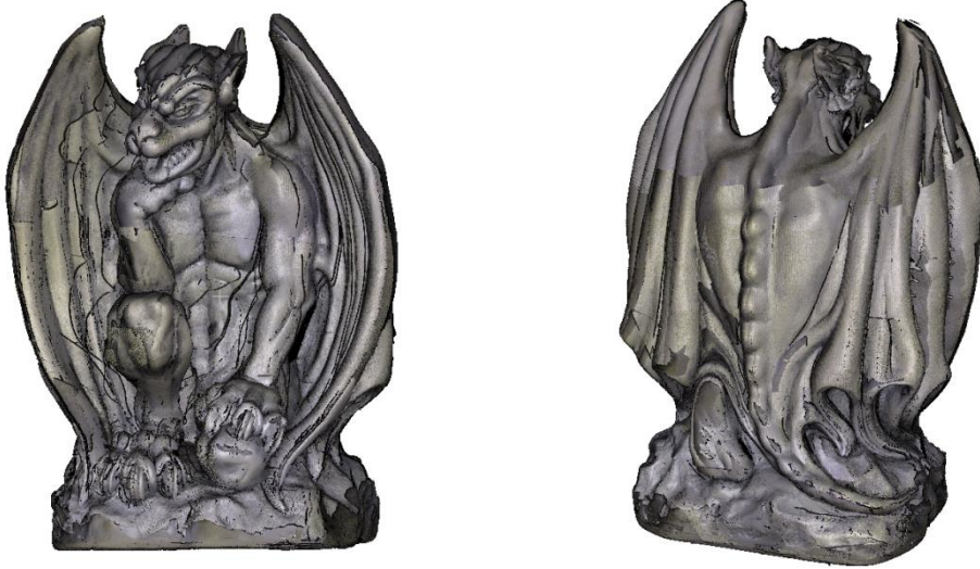
Figure 91. Rough 3D model of Gargoyle composed of 57 directional measurements.
