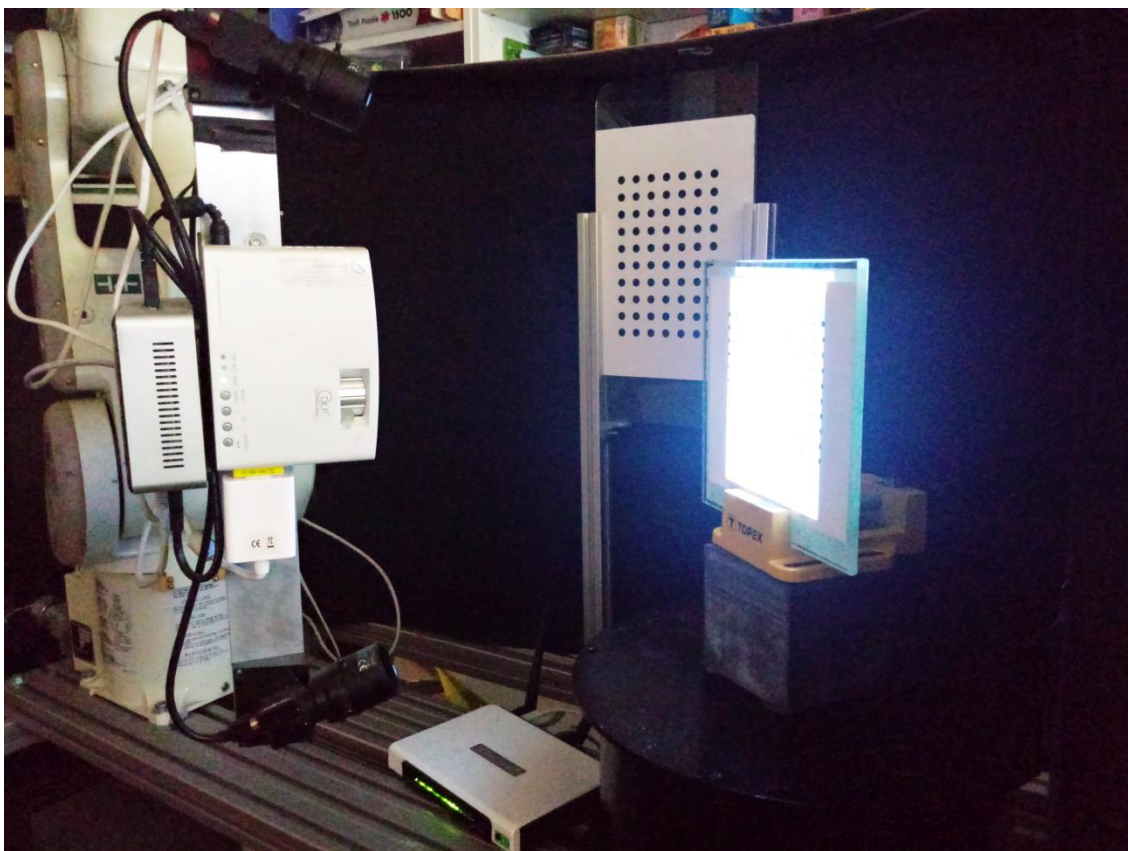
Figure 82. The digitization station used in the evaluation process. Custom-made 3D scanner for rough 3D scanning is fixed to robot arm.
