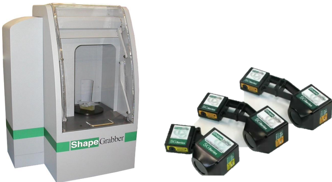
Figure 6. ShapeGrabber Ai310 (left) and its laser profilometers (right) (images source: ShapeGrabber website).
