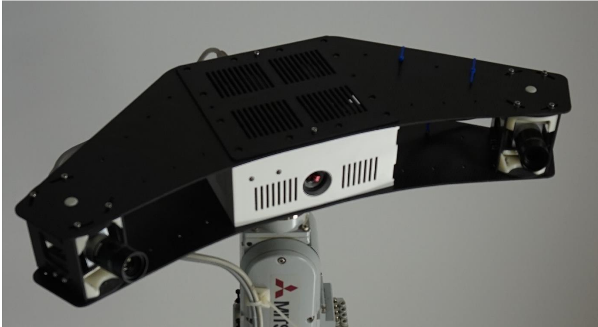
Figure 58. Measurement head with two CCD cameras.
