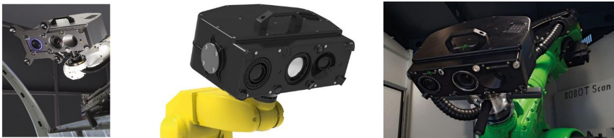
Figure 12. ZEISS Comet sensor on various robotic arms (image source: ZEISS Optotechnik webpage).
