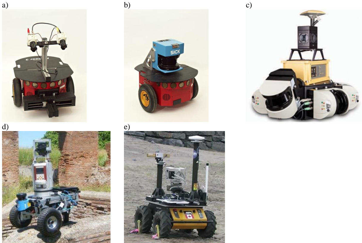
Figure 39. Mobile, ground-based 3D mapping platforms: a, b) Pioneer 3DX with stereovision (a) and rangefinder (image source: http://www.ti.uni-bielefeld.de ); c) Topcon IP-S2 Compact+ with multiple rangefinders (image source: manufacturers webpage ); d) custom platform with Riegl VZ-400 time of flight scanner; e) custom platform with time of flight scanner and rangefinders (image source: http://cyberspaceandtime.com ).
