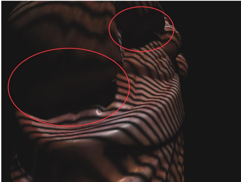
Figure 70. Occlusion during digitization process. Areas which cannot be digitized due to occlusion are marked with red ellipses.
