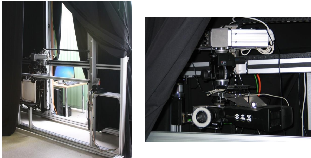
Figure 38. SAPO system with linear XY positioners (left) and its measurement head (right).
