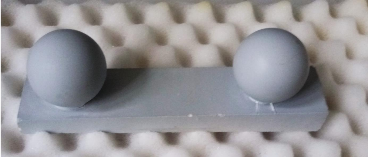
Figure 81. Test object (ball bar) used for assessing 3D sensor accuracy up to VDI/VDE standard.
