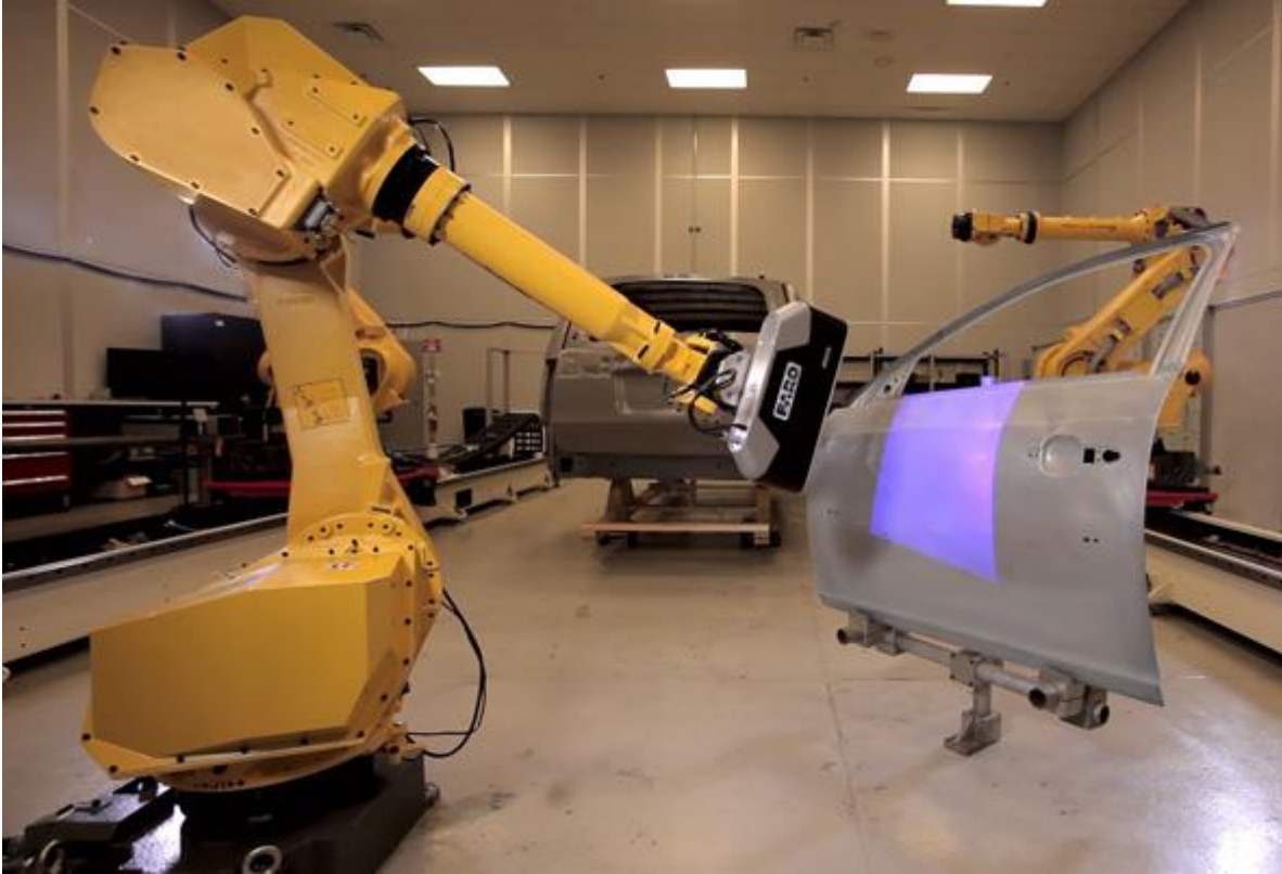
Figure 9. FARO Factory Array Imager (image source: FARO website).
