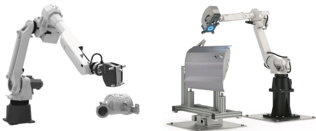
Figure 11. ZEISS T-Scan (left) and ZEISS Comet (right). Images source: ZEISS Optotechnik website.
