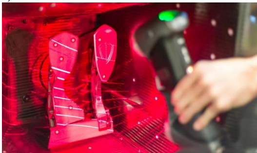
Figure 28. Typical laser triangulation system: (a) (b); with single laser stripe and rotating table providing movement of object (MakerBot Digitizer (MakerBot, 2016)) images source: MakerBot webpage; c) multi-stripe system (Creaform Handyscan (Creaform3D, 2016), image source: Creaform webpage); d) multi-stripe laser scanner (NextEngine), image source: NextEngine webpage.
