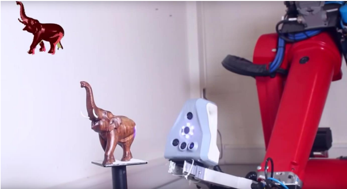
Figure 24. Artec Spider mounted to robot arm (image source: Artec 3D YouTube channel).
