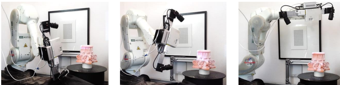
Figure 64. Predefined set of poses. For each robot configuration, table is rotated n times, by a 2\pi/n angle.
